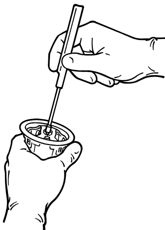
Figure 12. Insert the holder handle in the valve holder
