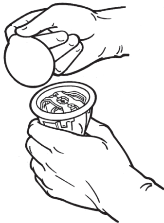
Figure 11. Remove the inner tray cover
