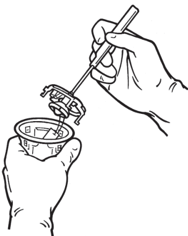
Figure 12. Remove the valve and collar from the inner tray
