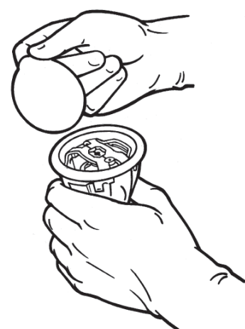
Figure 10. Remove the inner tray cover
