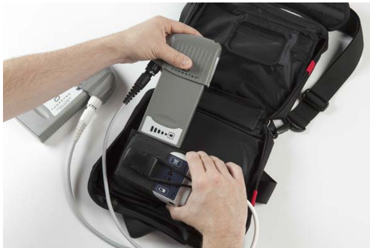
Figure 6.39 Place the Battery in the Bag
