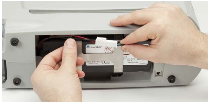
Figure 3.8 Fold the Wires and Connector Along the Top
