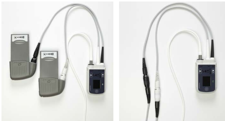
Figure 2.19 System Controller in Run Mode While on Battery Power (left) and the Power Module (right)
