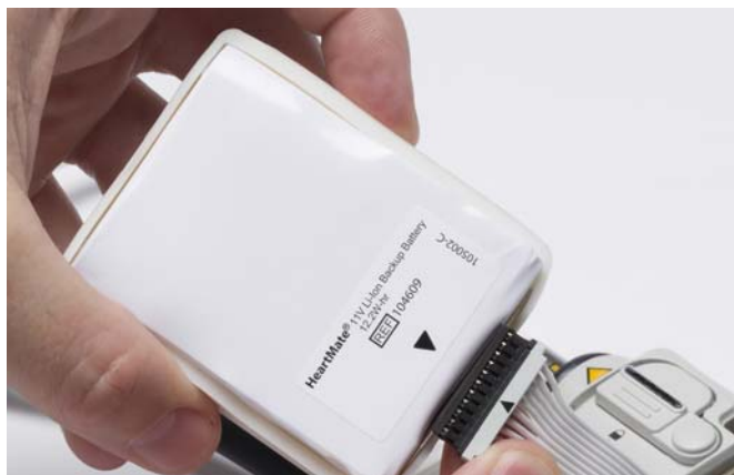
Figure 2.38 Install Backup Battery
