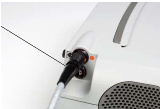
Figure 3.66 Tug on the Black Strain Relief Portion to Check the Connection
