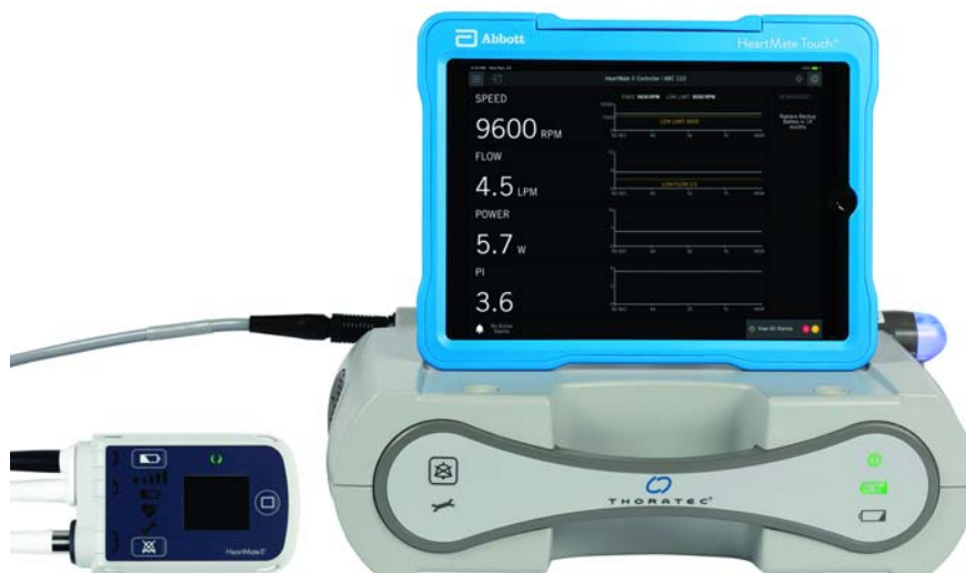
Figure 4.2 HeartMate Touch™ Communication System on top of the Power Module
