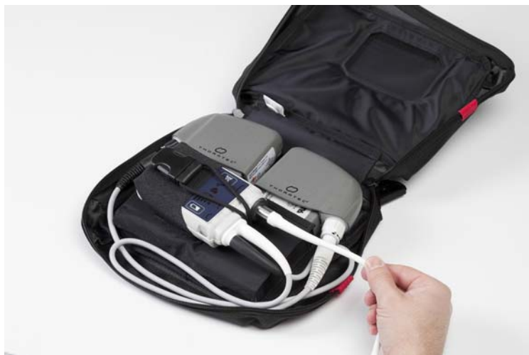
Figure 6.43 Close the Bag so the Driveline Exits Between the Red Tabs
