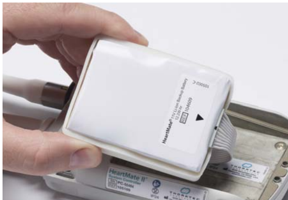
Figure 2.30 Place the Battery Inside the Battery Compartment
