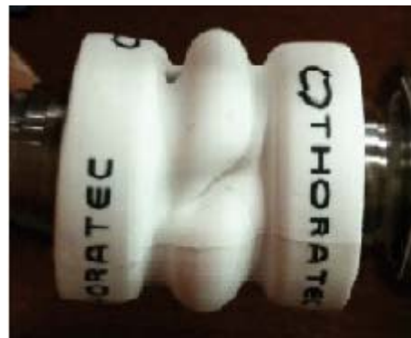
Incorrect: Twisted Silicone Sleeve
