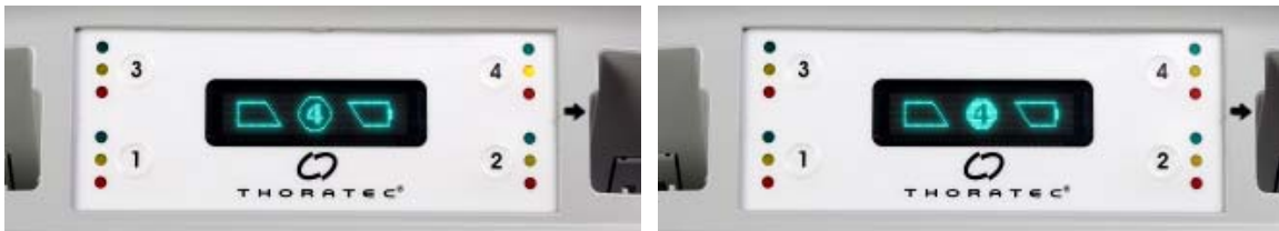
Figure 3.77 Calibration Prompt (in Graphic Mode) Indicates that the Battery in Pocket 4 Needs Calibration
