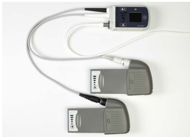
Figure 6.36 Make Sure the Power Cables and Driveline are Not Twisted
