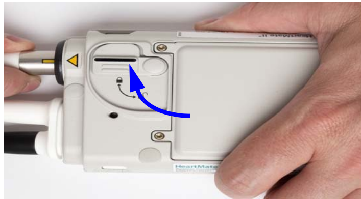
Figure 2.12 Insert the Driveline Into the Socket
