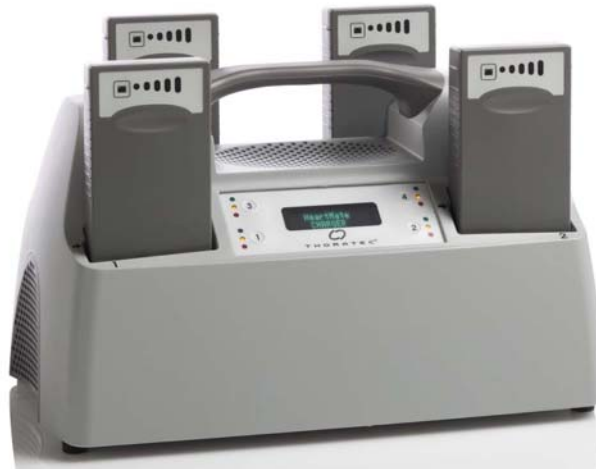
Figure 3.74 Batteries Inserted into Battery Charger Pockets
