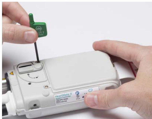
Figure 2.28 Use the Screwdriver to Loosen the Screws
