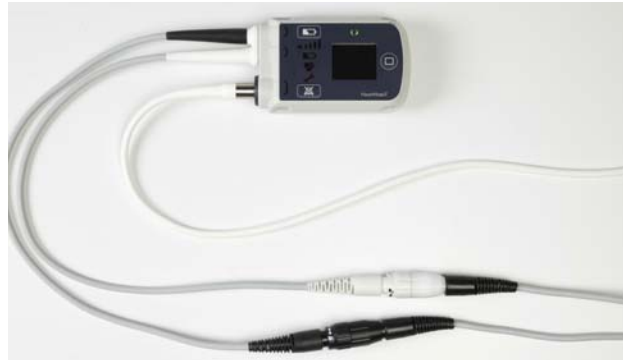
Figure 6.46 Make Sure the Power Cables and Driveline are Not Twisted
