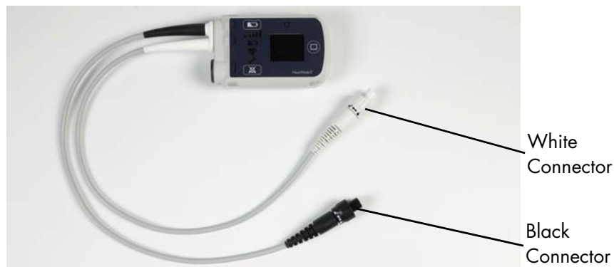
Figure 3.20 Black and White System Controller Power Cable Connectors
