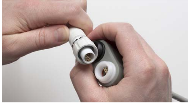
Figure 3.49 Carefully Align the Connectors
