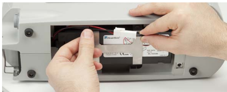
Figure 3.38 Gently Fold the Wires and Connector Along the Top
