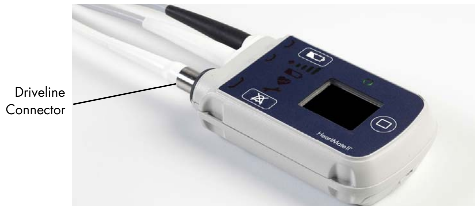
Figure 2.8 System Controller Driveline Connector
