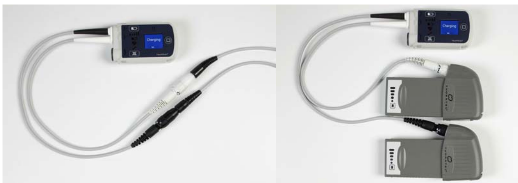
Figure 2.40 System Controller on Power Module Power (left) and Battery Power (right)
