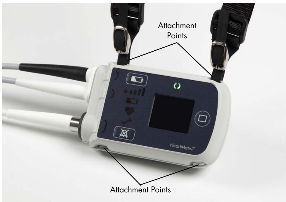
Figure 6.21 Attachment Points on the System Controller
