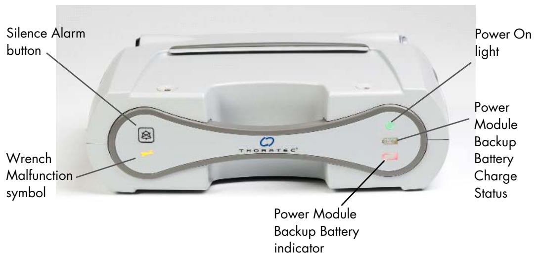
Figure 7.3 Alarm Indicators on Front of Power Module
