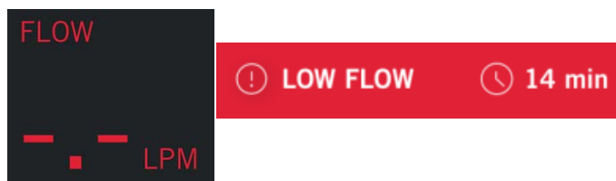
Figure 4.52 LOW FLOW Alarm and Pump Flow
