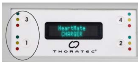
Figure 3.72 Press and Hold Buttons 1 and 3 to Change the Display Mode
