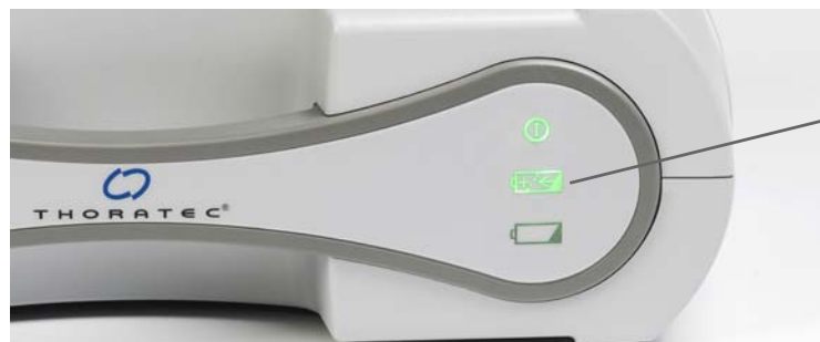
Figure 3.24 Green Charge Symbol Indicates that the Power Module Backup Battery is Charged
