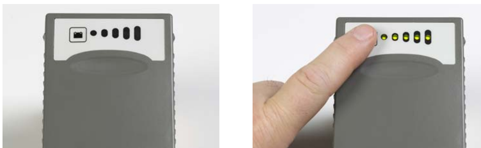
Figure 3.58 On-Battery Power Gauge: Press Battery Symbol to Activate Bars
