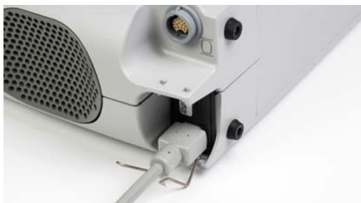
Figure 3.10 Plug the Power Cord into the Power Module
