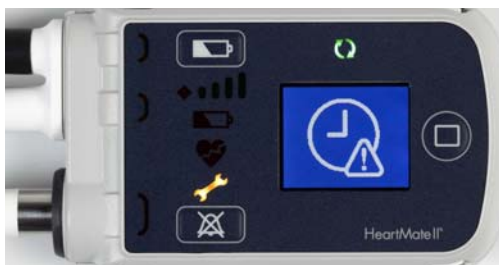
Figure 2.32 System Controller Clock Not Set Advisory Alarm
