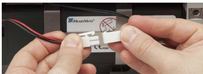
Figure 3.37 Line Up the Connector Halves
