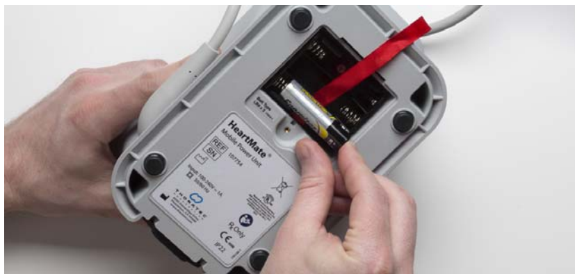
Figure 3.43 Install AA Batteries
