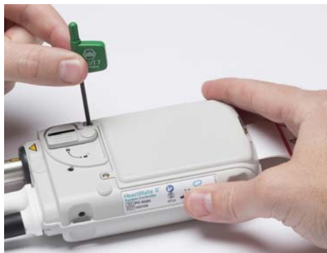
Figure 5.31 Use the Screwdriver to Loosen the Screws
