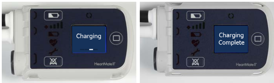
Figure 2.23 System Controller Charging or Charging Complete
