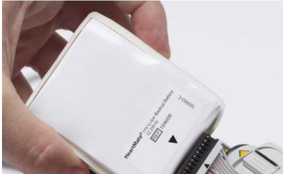
Figure 2.29 Remove Ribbon Cable from Battery Socket
