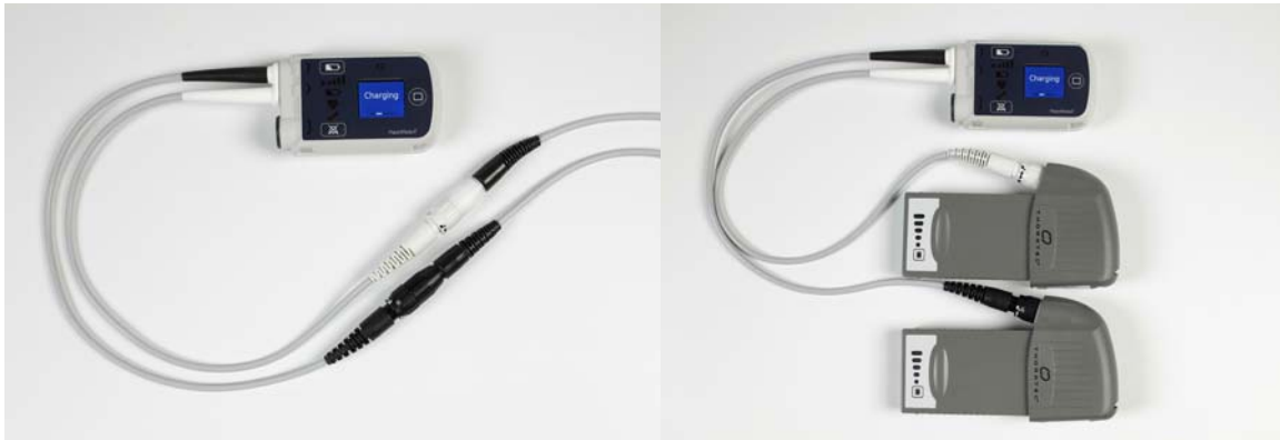
Figure 2.21 System Controller in Charge Mode
