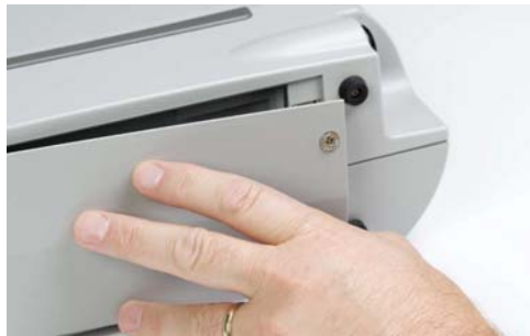
Figure 3.3 Remove the Battery Compartment Cover
