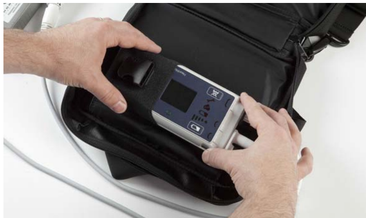
Figure 6.37 Slide the System Controller Into the Holder in the Consolidated Bag
