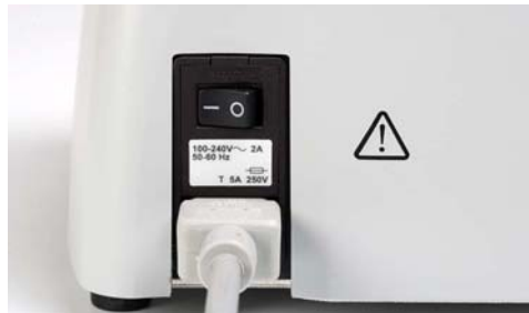
Figure 3.68 Plug the Power Cord Into the Battery Charger
