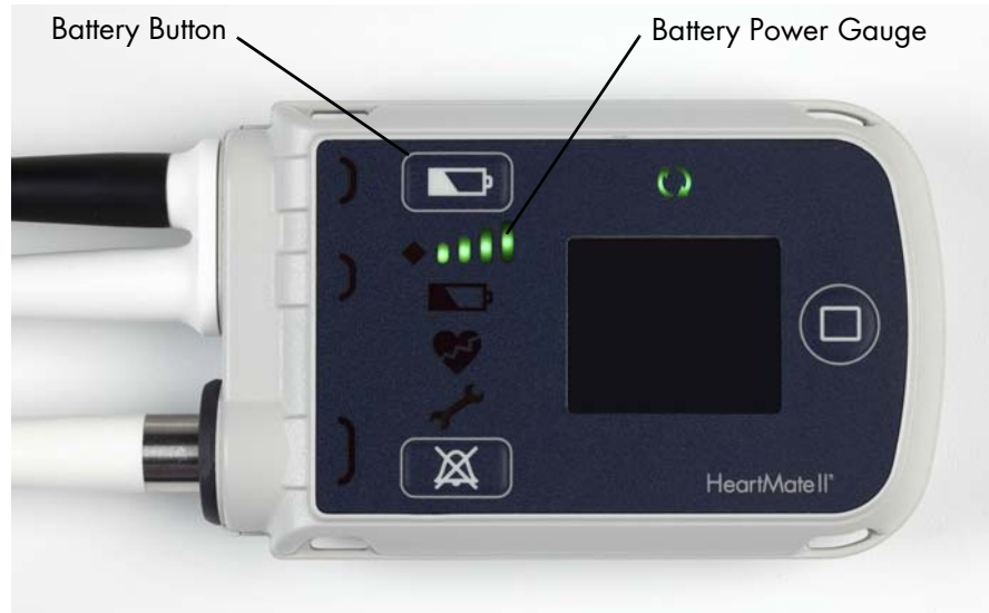
Figure 2.18 Battery Power Gauge Showing Full Charge
