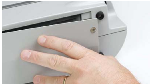
Figure 3.35 Remove the Battery Compartment Cover
