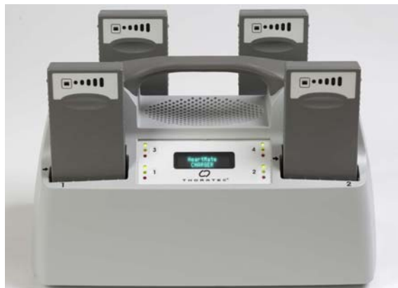
Figure 3.76 Battery Charger with Batteries Inserted in All Pockets
