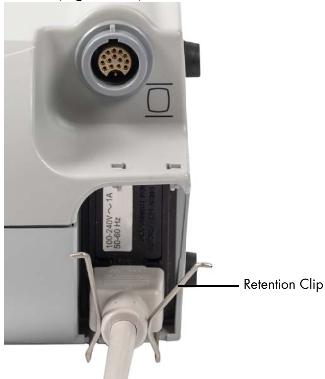
Figure 4.4 Disengage the Retention Clip
