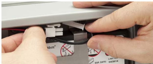
Figure 3.36 Gently Pull the Wires and Connector Halves Out
