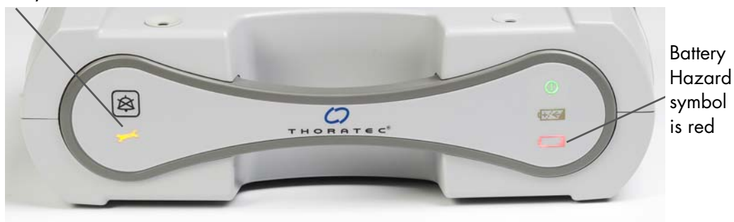
Figure 3.27 Yellow Wrench and Red Battery Hazard Symbol Indicate that the Power Module Backup Battery is Not Working — Switch to Another Power Source Immediately
