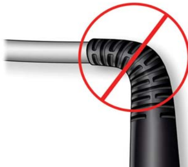
Figure 6.61 Do Not Bend System Controller Power Cables
