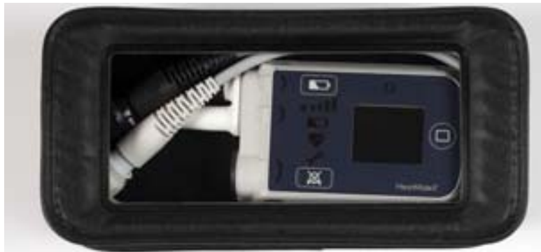
Figure 6.57 Protection Bag with Backup Controller and Cables Stored Inside
