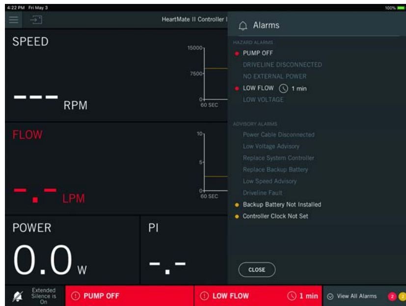
Figure 4.46 Alarms Panel with Multiple Active Alarms
