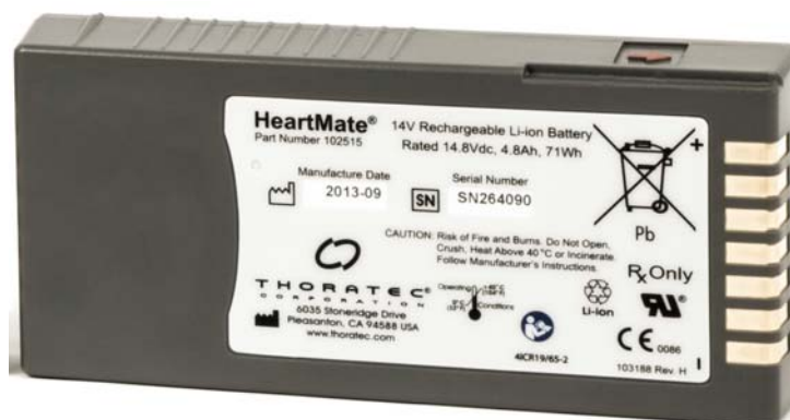
Figure 3.54 HeartMate 14 Volt Lithium-Ion Battery
