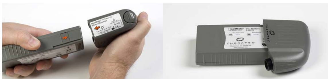
Figure 3.55 Inserting Battery into Battery Clip
