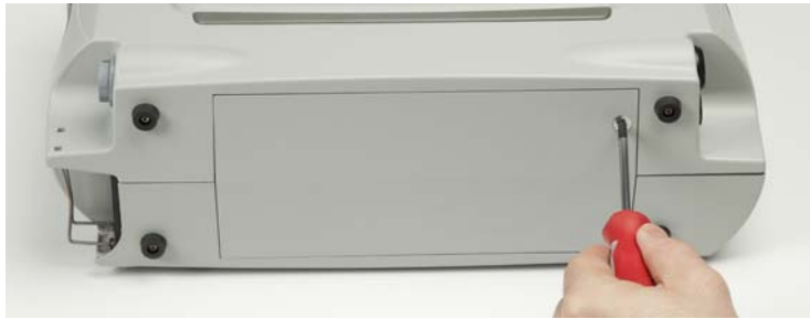
Figure 3.2 Loosen the Screws
