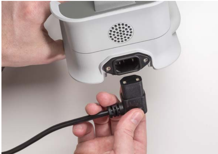
Figure 3.45 Plug Power Cord into Mobile Power Unit
