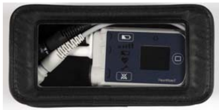
Figure 2.43 Backup System Controller in Protection Bag
