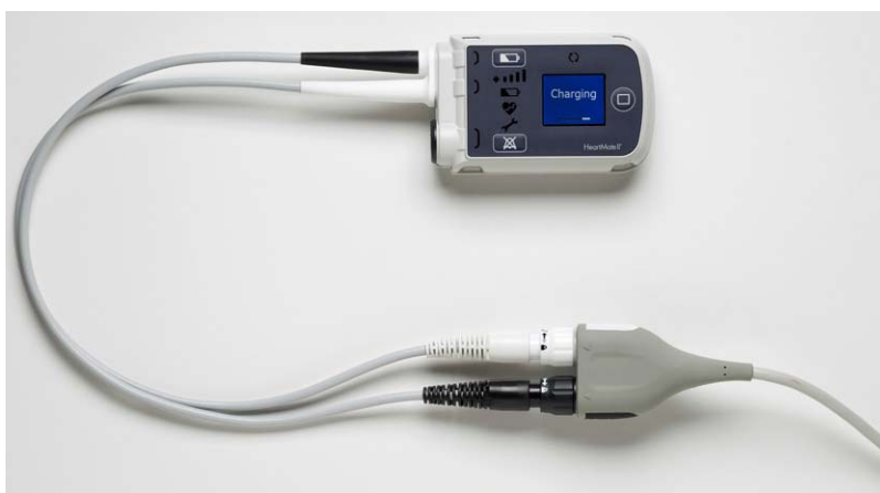
Figure 3.52 System Controller Power Cables Connected to Mobile Power Unit Patient Cable Connectors
