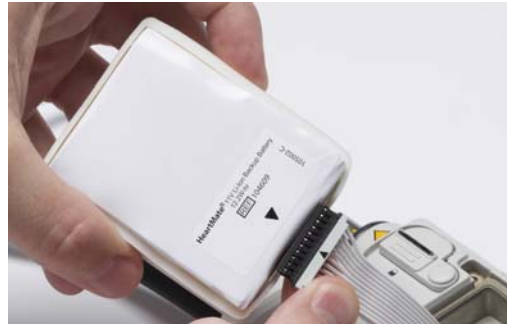
Figure 5.32 Align the Arrow on the Cable with the Arrow on the Battery
