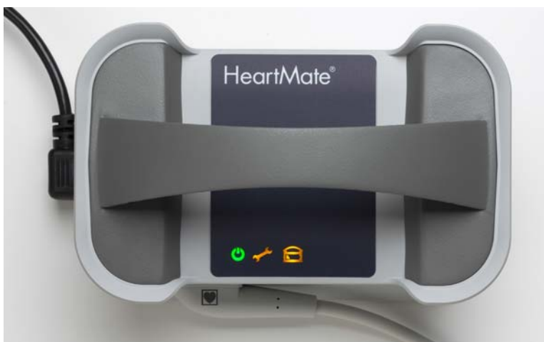
Figure 7.4 Indicators on the Mobile Power Unit
