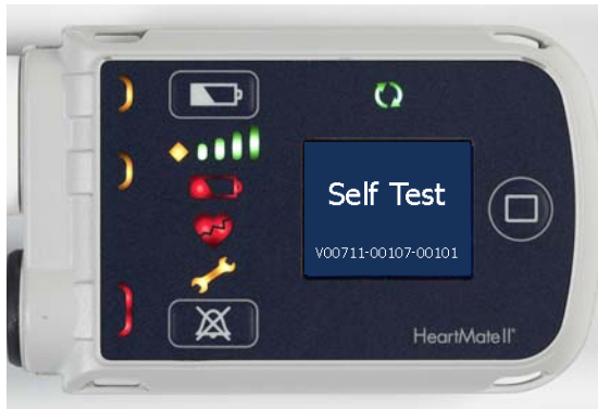
Figure 2.17 User Interface During System Controller Self Test
