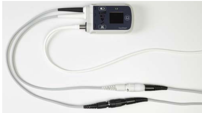
Figure 6.23 Make Sure the Power Cables and Driveline are Not Twisted
