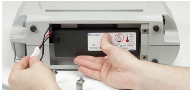
Figure 3.6 Place the Battery in the Battery Compartment
