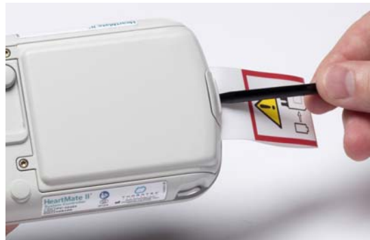
Figure 5.30 Use the Lever to Remove the Screw Cover
