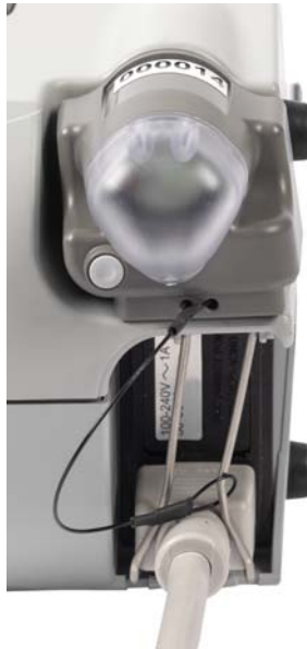
Figure 4.7 Insert the HeartMate Touch™ Wireless Adapter into the Power Module Socket
