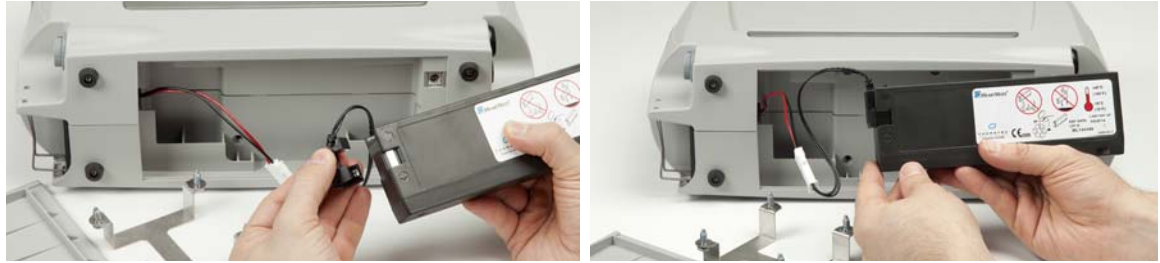
Figure 3.5 Secure the Battery to the Battery Connector
