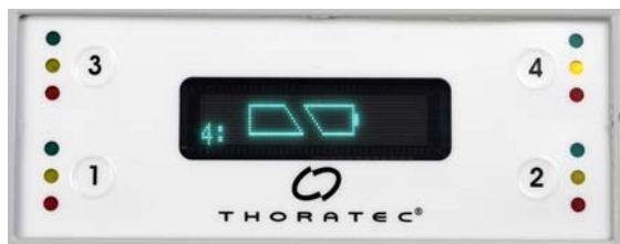
Figure 3.78 Calibration Status Screen Indicating that Battery in Pocket 4 is Being Calibrated
