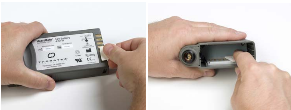
Figure 8.1 Clean the Battery Contacts and Clips
