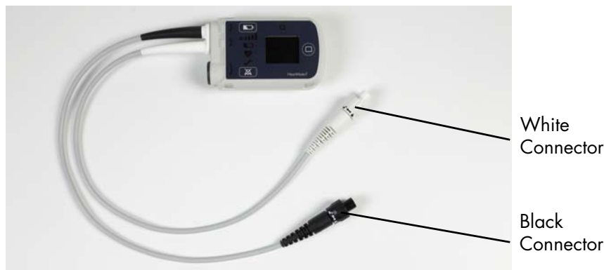
Figure 3.48 System Controller Power Cable Connectors
