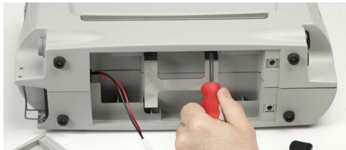
Figure 3.4 Remove the Metal Bracket
