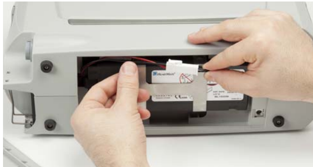
Figure 3.30 Gently Pull the Wires and Connectors Away
