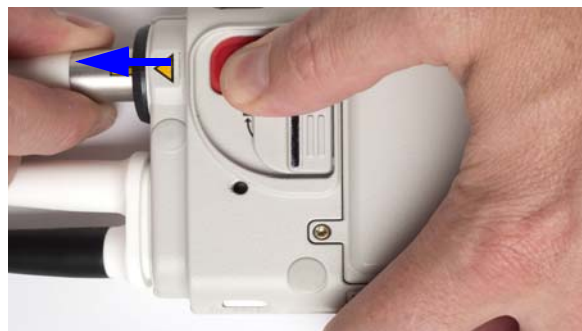
Figure 2.14 Grasp the Metal End and Remove the Driveline
