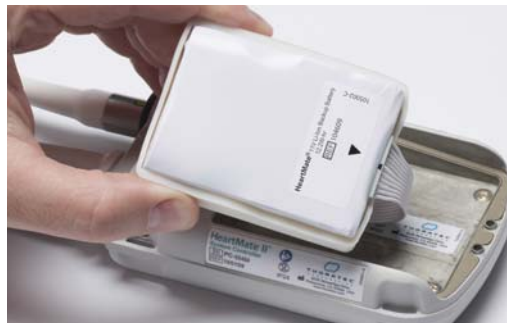
Figure 5.33 Place the Battery Inside the Battery Compartment
