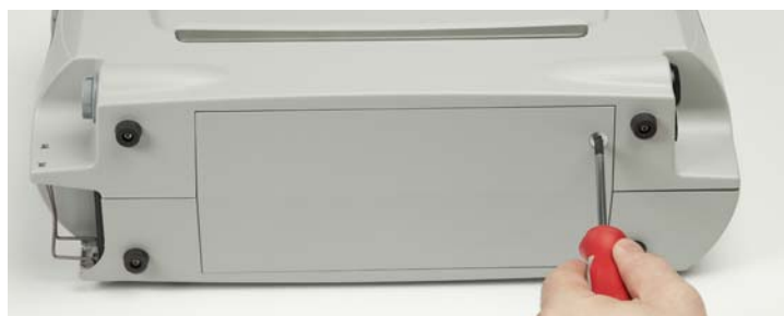
Figure 3.28 Loosen the Screws
