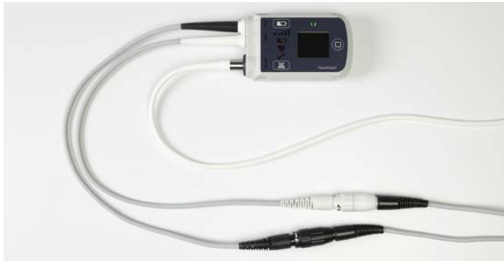
Figure 3.23 System Controller Power Cables Connected to Power Module Patient Cables
