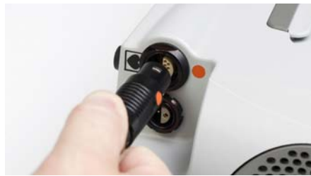
Figure 3.19 Align the Red Dot on the Connector with the Red Dot on the Power Module
