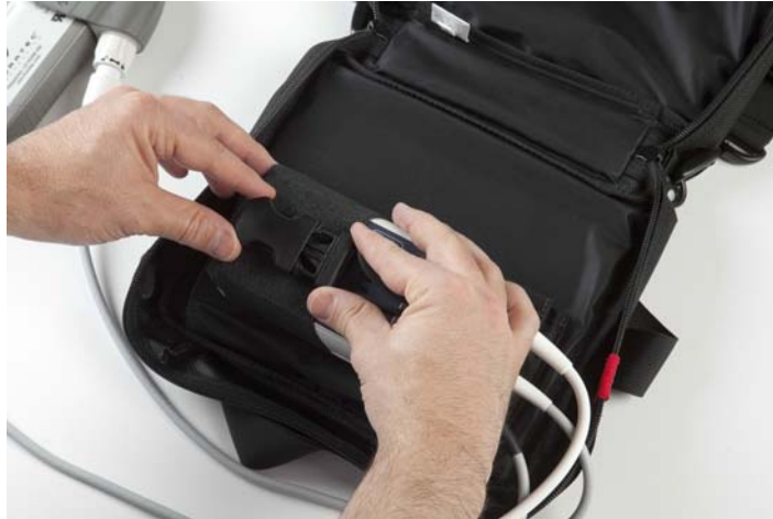
Figure 6.38 Stretch the Strap Over the System Controller and Between the Cables
