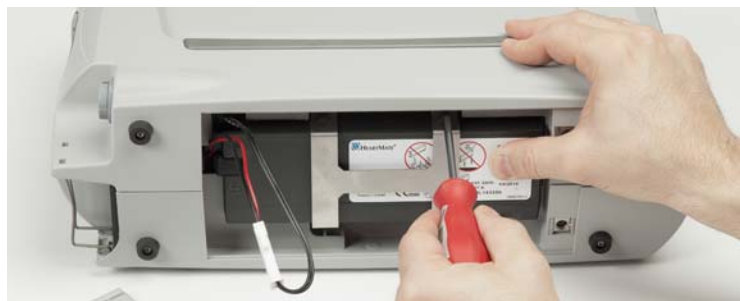
Figure 3.7 Reattach Metal Bracket
