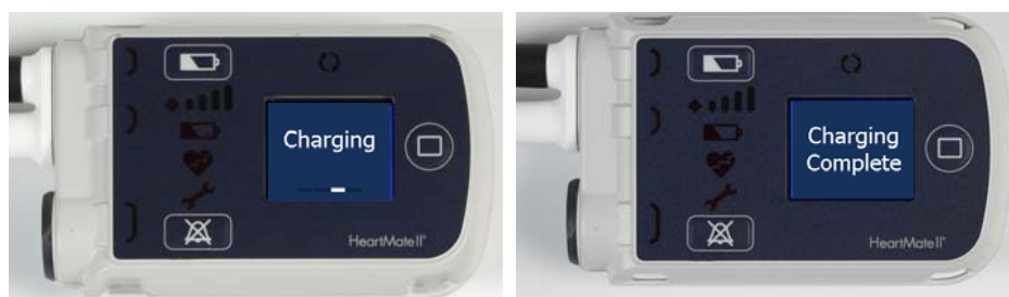
Figure 2.41 System Controller Charging or Charging Complete
