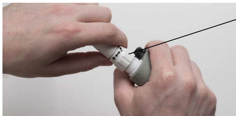
Figure 7.7 Turn Nut on the Connector
