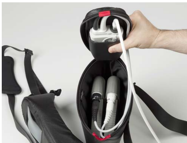
Figure 6.10 Position the Power Cables Inside the Bag
