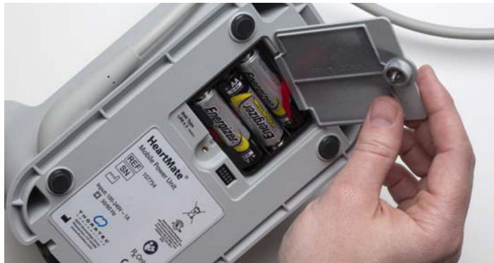
Figure 3.42 Remove the Battery Compartment Cover
