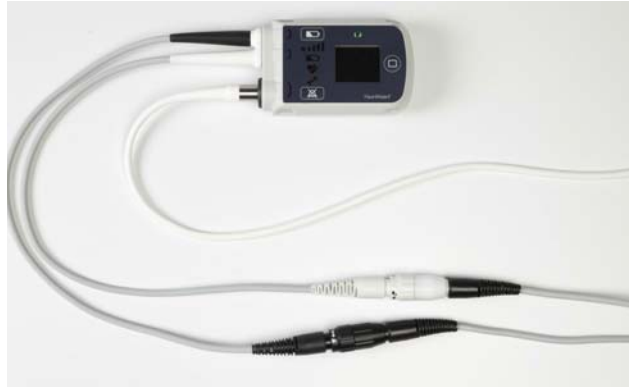
Figure 6.52 Make Sure the Power Cables and Driveline are Not Twisted
