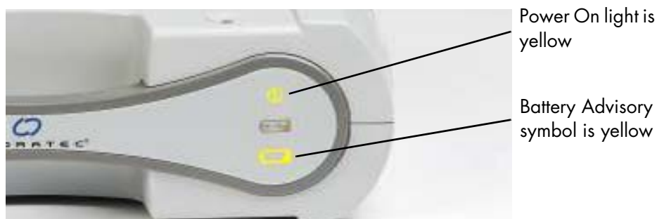
Figure 3.26 Less than 15 Minutes of Power Module Backup Power Remain When Power On Light and Battery Advisory Symbol are Yellow
