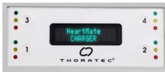
Figure 3.75 Charge Status Lights (Green, Yellow, Red) for Pockets 1 through 4
