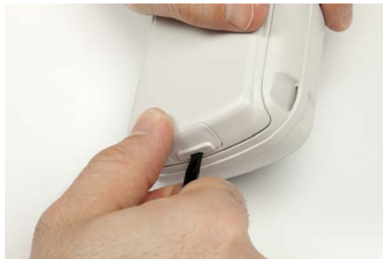
Figure 2.27 Use the Lever to Remove the Screw Cover
