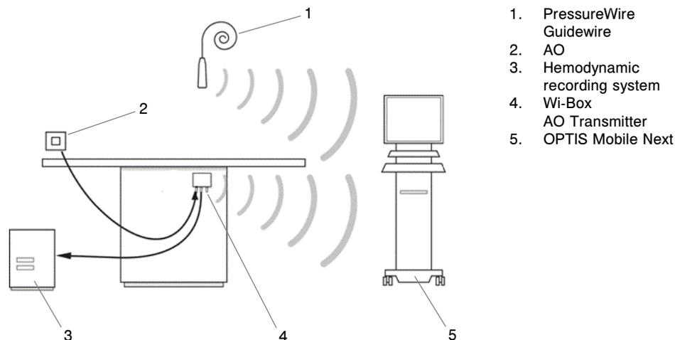
The wireless connection to the Wi-Box AO Transmitter is made during setup for the procedure. Refer to the installed software User Manual for more information.
